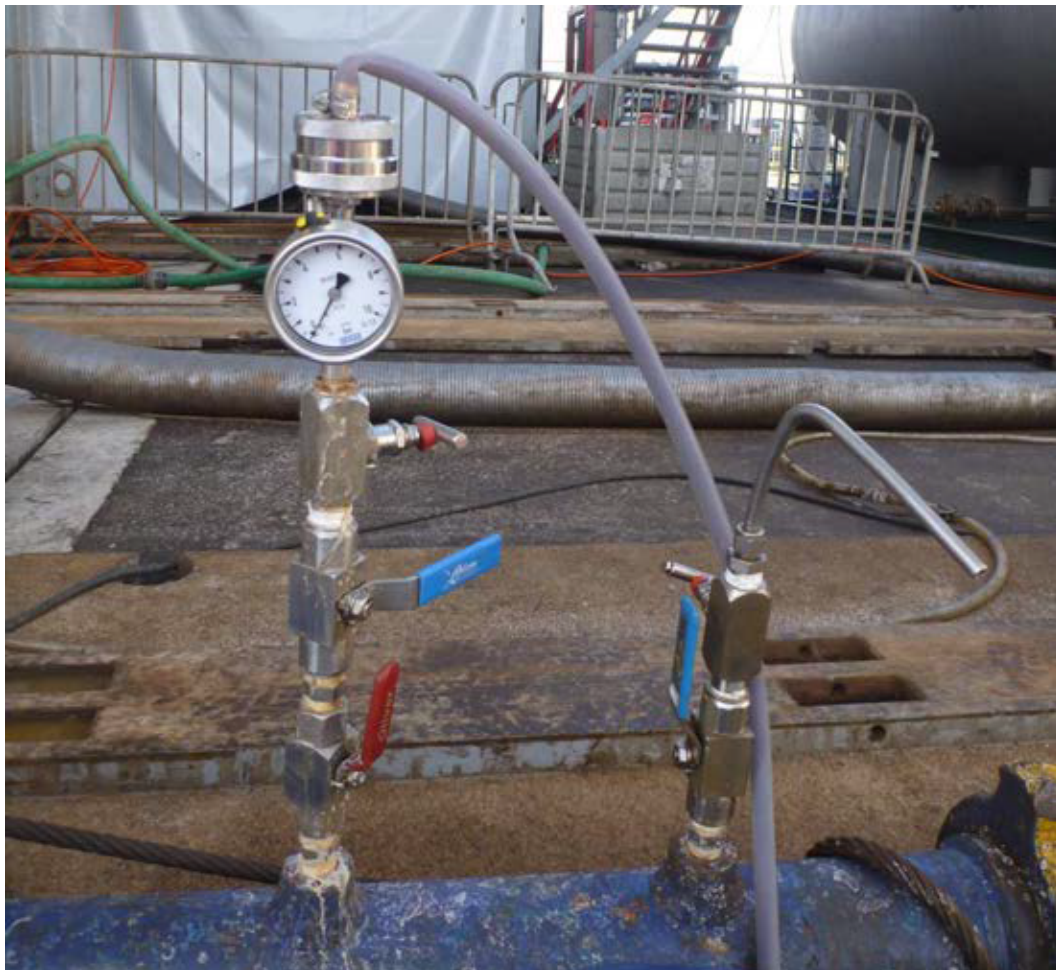
Figure 8: Filtering device at drillsite Honselersdijk consisting of ball values, feed regulator, pressure gauge and a cross flow sampler on top.
