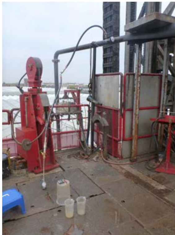
Figure 8: Filtering device at drillsite Honselersdijk consisting of ball values, feed regulator, pressure gauge and a cross flow sampler.
